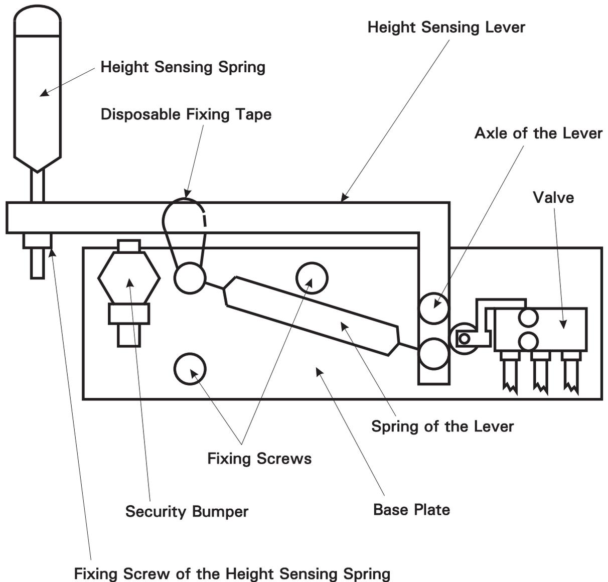
If there is any adjustment seems to be necessary, only the Fixing Screw of the Height Sensing Spring should be opened, and the Height Sensing Spring should be turned into another position. After making the modification the Fixing Screw should be closed again.
