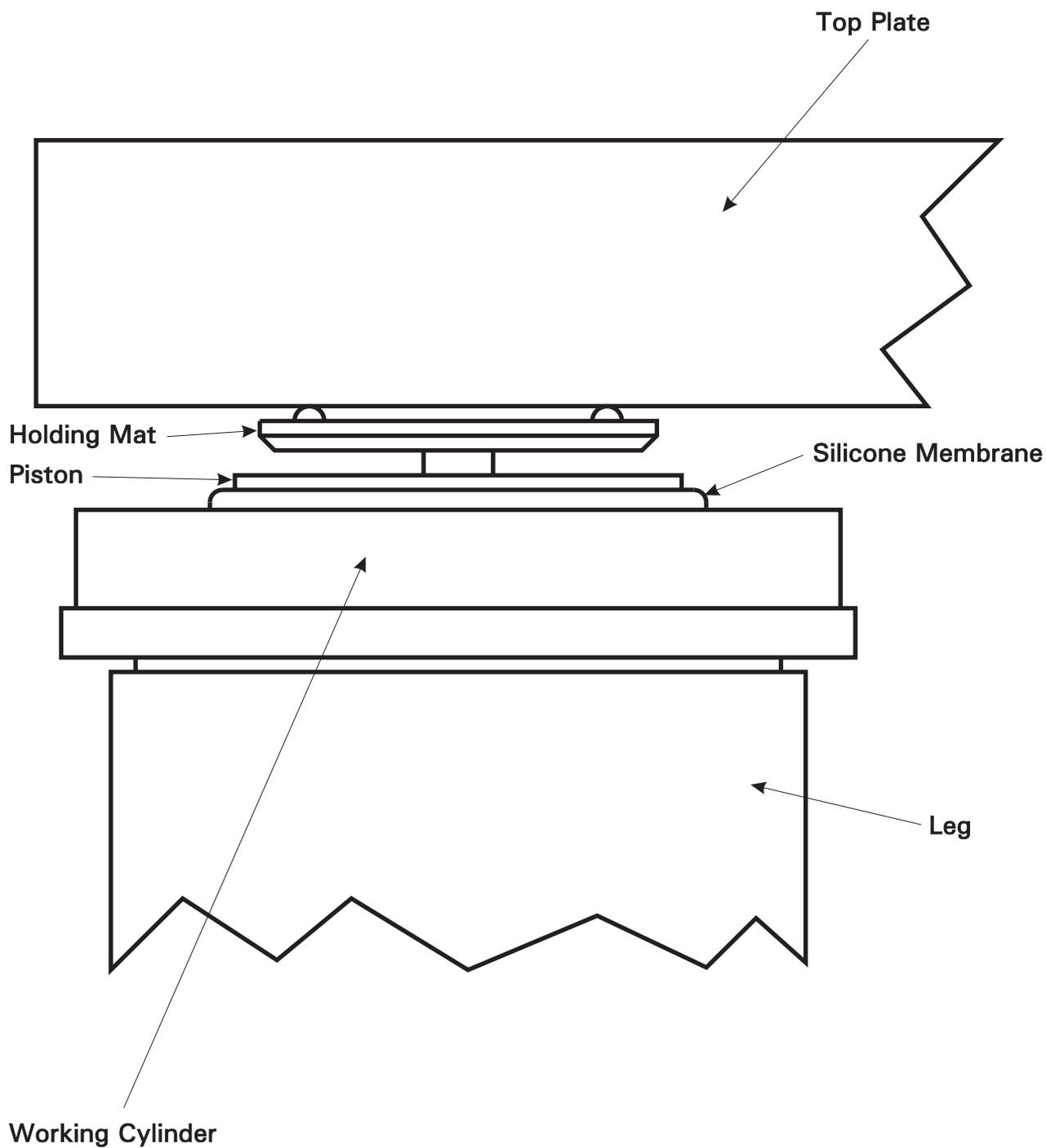
**Figure 2. Parts of the Working Cylinder (Small Table)**
