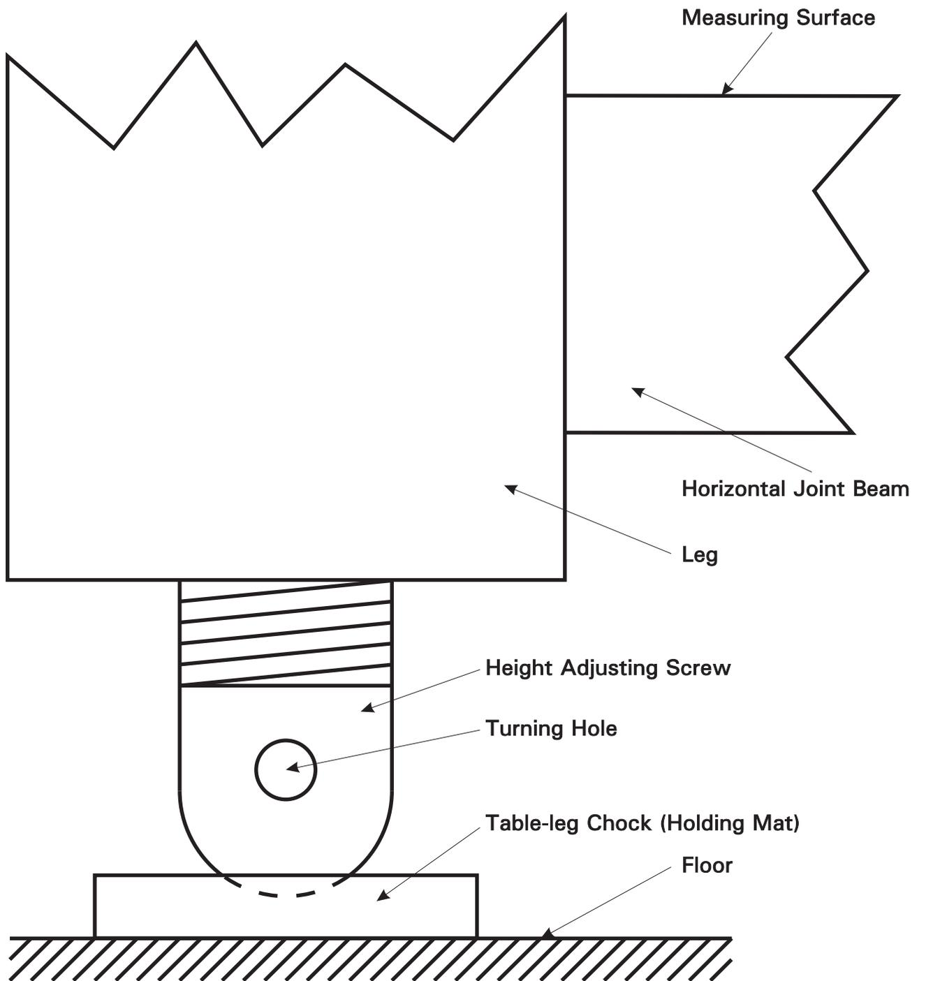
**Figure 1. Horizontal level adjustment of the leg system**
