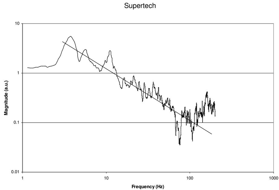
This graph shows the worst case attenuation, because it was measured on the smallest vibration isolation table SUPERTECH Instruments manufactures. The bigger sized tables have better attenuation, proportional to their size.
