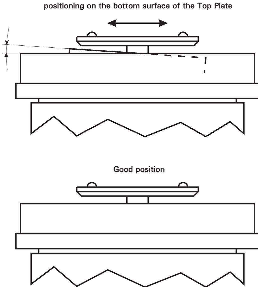
**Figure 5. Positioning of the vertical angle of the Piston in the Working Cylinder of the Small Tables**
