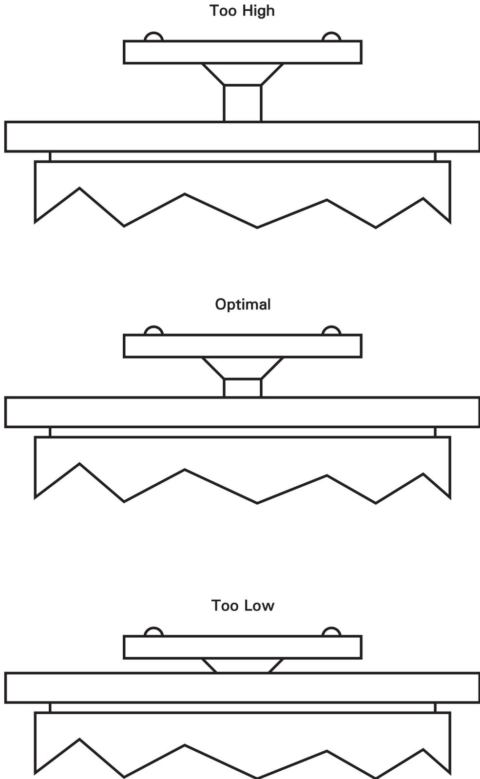
**Figure 6. Adjusting the height of the Piston in the Working Cylinder of the Large Tables**
