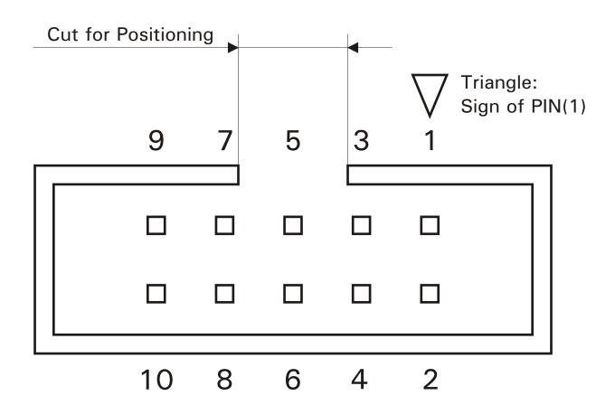
Input Connector of the 4-channel Differential Preamplifier of the DC BioAmp V7.2
