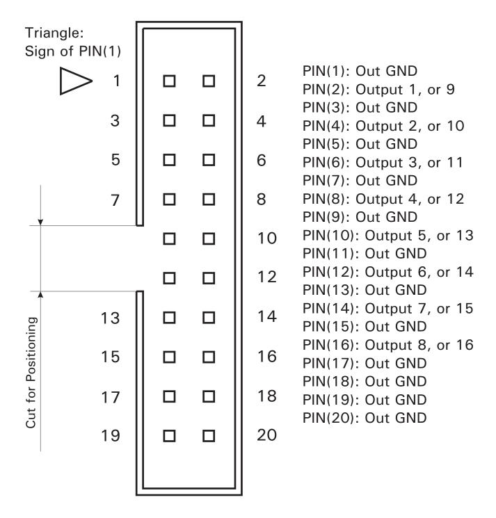
The appropriate 20-pin, 2.54 mm female plug compatible with this output connector is IDS-020-S100-01/P manufactured by E-tec Corp.
