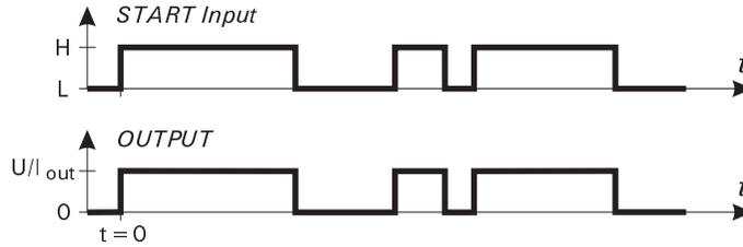
Output is active, while START button is pressed, or TTL high level is applied to START Input. This mode offers free control capability from any other equipment (e.g. another stimulator controller, or a TTL port bit of a computer).
