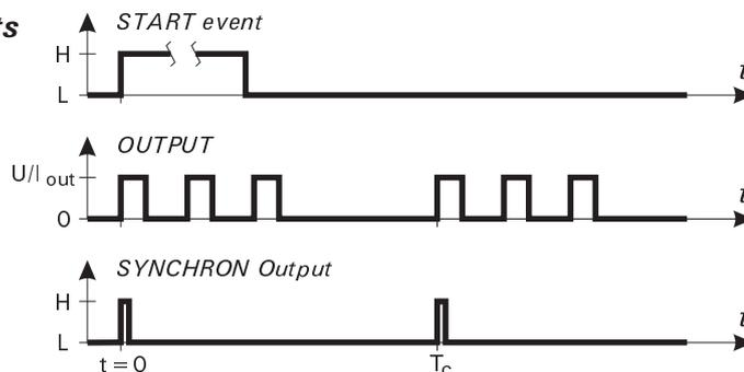
Repetitive bursts of pulses (2 - 99 pulses/cycle) are generated on the Output. The time parameters of the components in the bursts are the same as in the Single Burst, and the Delayed Burst functions. The repetition cycle time (Tc) can be set from 10 ms - 60 sec, with 10 ms of resolution. A Synchron pulse is generated at the rising edge of the first Output pulse (once at the beginning in every bursts).
