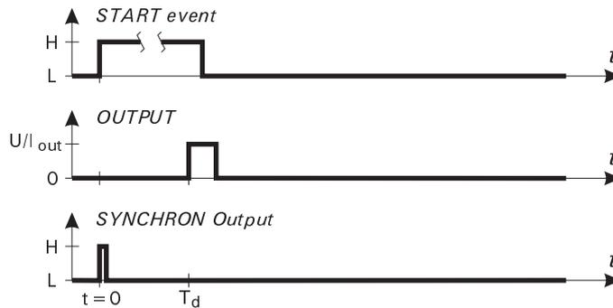
A delay (1 - 250 milliseconds in width, with 1 ms of resolution) is occurring after START event. Just after the delay time an Output pulse is generated (0.1 - 9.9 milliseconds in width, with 0.1 ms of resolution). A Synchron pulse (50 μs) is generated at the START event (at the beginning of the delay time period). Single Pulse function is a special case of Delayed Pulse function, when delay time equals to zero.
