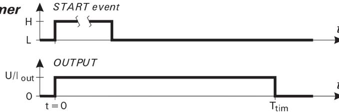
Output is active (constant DC level adjustable by the helical potmeter on the End-stage) in a programmed period, in the range of 10 - 600 sec, with 10 sec of resolution. This period starts at the beginning of the START event.
