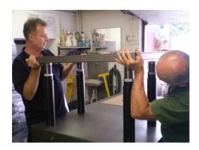
For the fixation of the plate 4 pieces of M6 inbus screws are needed. At first, strain the screws together with the M6 steel holding mats into the holes of the legs only slightly so you can adjust the top plate to its proper place too.
