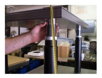
After having made the proper adjustments, strain the inbus screws until fixed. Finally, strain the 2 inch lock nuts manually so they're tight and your table is ready.
