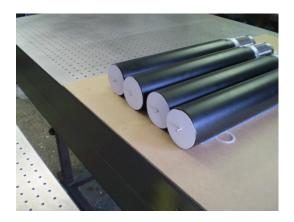
Then screw the legs into the M6 holes of the table into their desired places, strain them manually and put paper holding mats on the top of the legs as well. When all four legs are at their appropriate places, adjust them to the same height with 2 inch adjustable screws.
