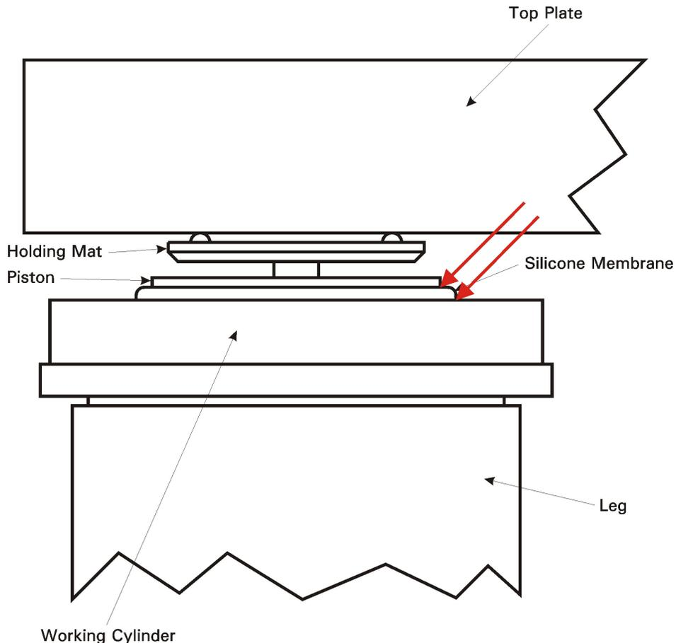
In case of finding an injured membrane all the working cylinders should be changed (one is faulty and the other three pieces as preventive renewing). This task needs a lifting trolley, because the top plate should be removed from the legs. A broken membrane is very rare case, during normal operation the membrane nearly works for eternity. Most of the time a membrane blows up during an improper installation.
