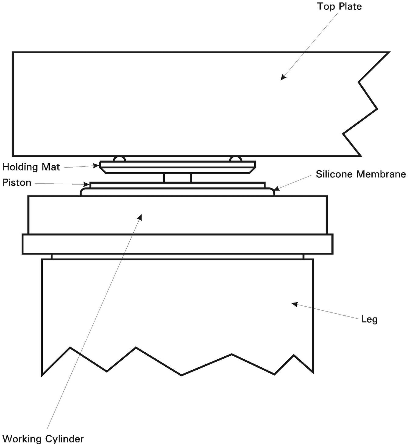
The air should be completely let out from the working cylinders by lifting the height sensing levers. Then, after releasing the air from the working cylinders, the height sensing levers should be fastened to the security bumpers by rubber O-rings or fixing tape. It is important because this way, when moving the top plate on the lifting trolley, the height sensing springs and levers will not be damaged.
